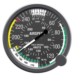
The picture is of a classic "steam gage" airspeed indicator that also has True airspeed scales, which is a little unusual. (The white scales). Neither of the club planes altimeters has the True airspeed scales.
