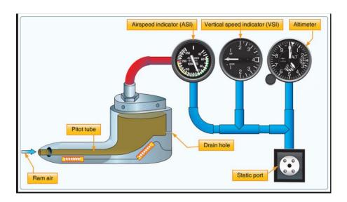
The picture shows the Pitot tube connected to the airspeed indicator and the static air pressure vent port connected to the airspeed, vertical speed and altimeter, which is correct. Right now we're just interested in the airspeed indicator.
